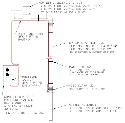
FOR CONNECTION TO WATER SYSTEM WITH NO ELECTRIC START/STOP (SUCH AS CITY WATER SUPPLY):
