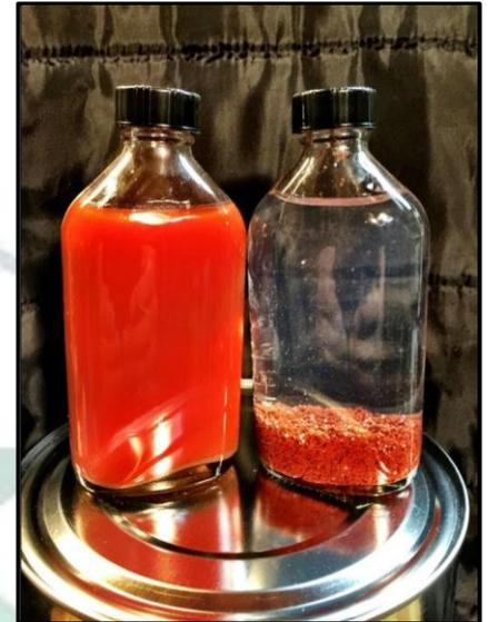
You may add SlurryDry™ to the remaining thickened sludge material to dehydrate the remaining moisture and creating a safe material for standard disposal that meets the requirements for the EPA 9095B Paint Filter Test for adequate moisture levels.
