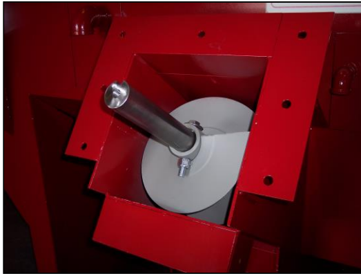
A Drive Shaft installed using (2) 5/8" Grade 2 Hex Head Cap Screws and associated hardware.
