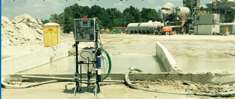
CO<sub>2</sub> gas is available virtually everywhere, through your local gas or welding supplier. It is considerably safer and less expensive then sulfuric and hydrochloric acid.
