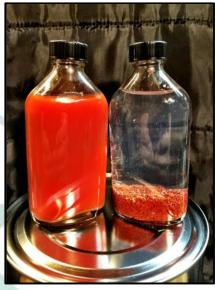
You may add SlurryDry™ to the remaining thickened sludge material to dehydrate the remaining moisture and creating a safe material for standard disposal that meets the requirements for the EPA 9095B Paint Filter Test for adequate moisture levels.
